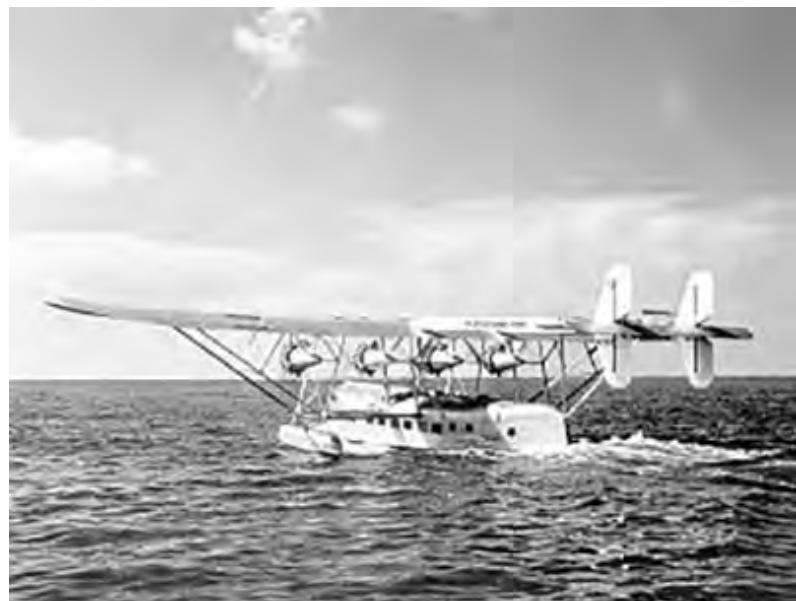
A Sikorsky S-40 was the aircraft that they planned on using. Only three were actually built at a cost of 250 thousand dollars each for Pan American World Airways. It seated 38 passengers as opposed to the S-38, which only carried eight and was probably the aircraft that they eventually purchased – too little and too late. Given the size of their budget, just the cost of the original aircraft would have probably doomed their scheme.
