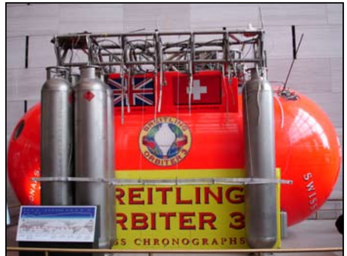
Photo showing the side view of the Breitling Orbiter III gondola. Note: as the fuel was consumed the empty tanks were dropped over unpopulated areas. This practice lightened the load and conserved fuel consumption.
