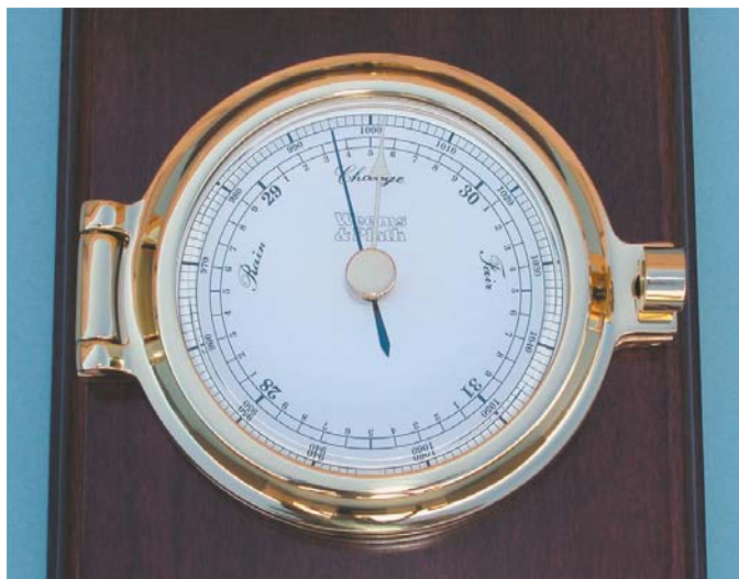
Figure 7. Household Aneroid Barometer.
