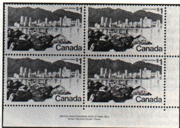
Fig. 10. BABNC 'harrow' perforation. Note the misalignment caused by a bent pin in the fourth hole from the right margin in the bottom row of horizontal perforations.
